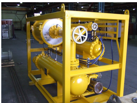
The Infinity Supercritical SDR1200 can process 1,200 kilograms of botanicals per day. Dual flow redundancy allows seamless operation.
